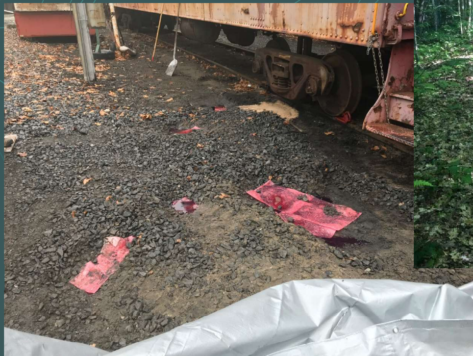
Oil drippings (spill?)
